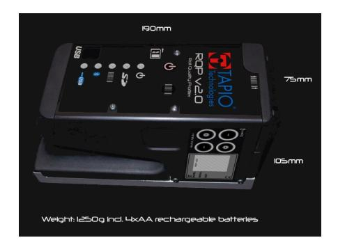
TAPIO RQP v2.0 measurement is based on a position measurement. The penetration of the hammer is also measured providing new interesting information about the measured surface. The absolute values do not differ between different measurement units.
